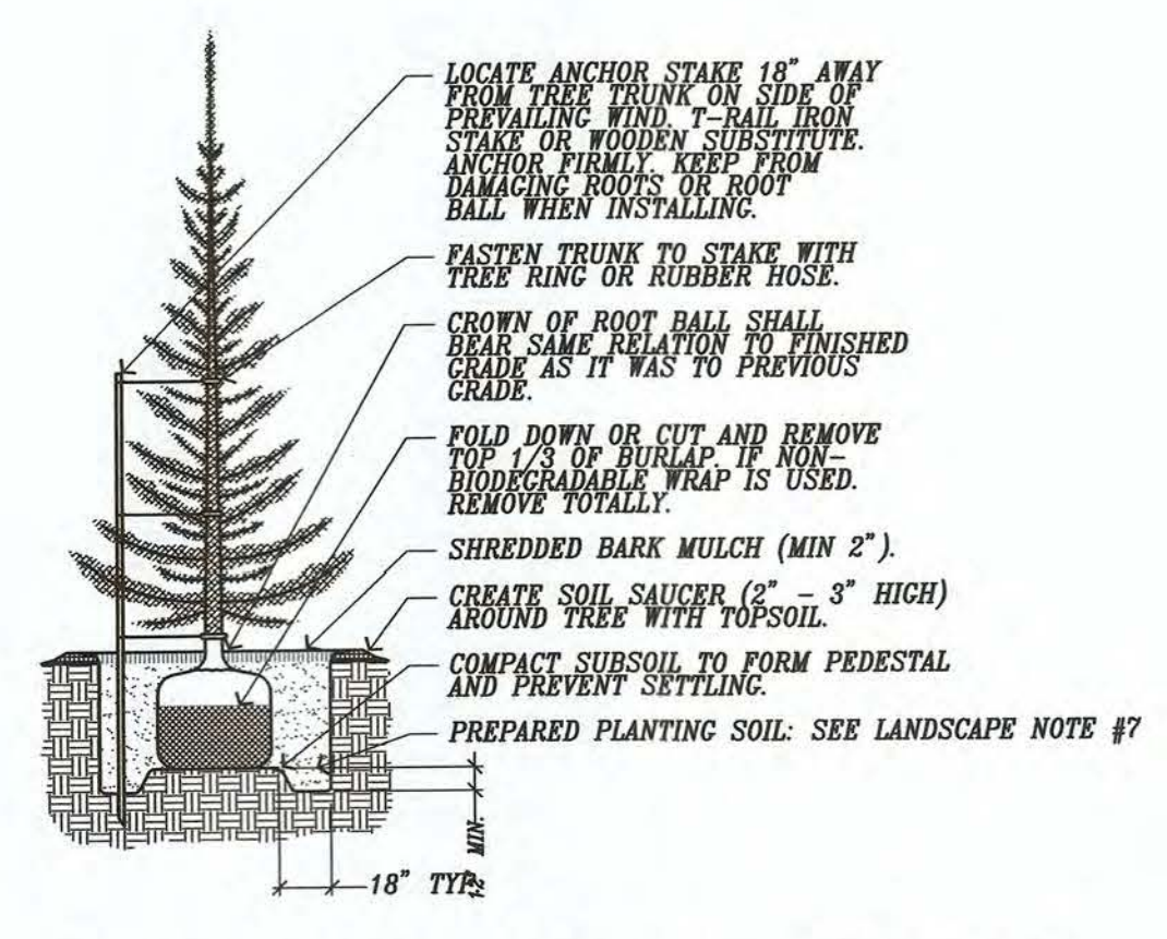
8 CONIFEROUS TREE PLANTING DETAIL N.T.S. FILE:
